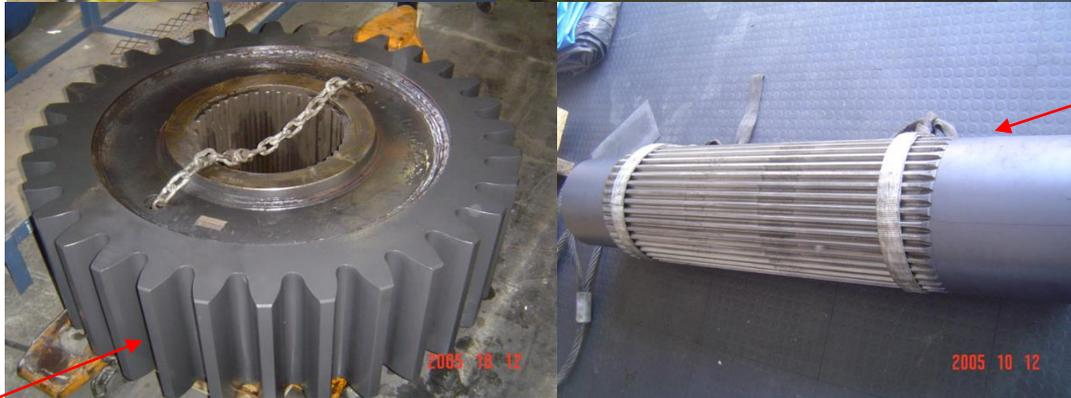
The processed steel used in this main shaft proved to be flawless, hence the perfect Cryogenic Thermal Treatment Process. The Main Shaft was also then CermaLube Dry Film Lubricant Coated.
